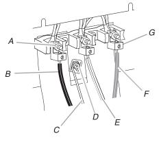
A. 10–32 hex nut B. Line 1 (black) C. Bare (green) ground wire D. Ground-link screw
